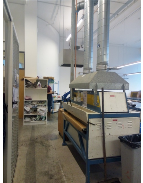
Figure 3: Heat press with overhead exhaust system. They are planning to shift it against the wall in place of the shelf due to its inconvenient location.
